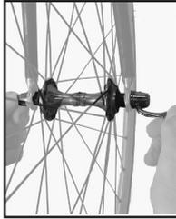
Figure 3- Wheel quick-release
