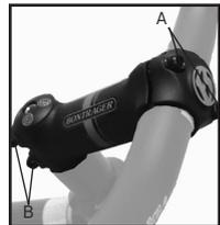
Figure 11- Direct-connect stem
