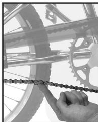
Figure 6- Checking chain tension
